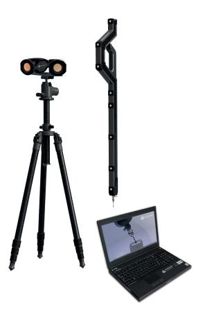
Metronor SOLO Twin uses two separate cameras to generate each image. By effectively doubling the field-of-view, the camera can be placed closer to the measurement object, increasing accuracy and enabling measurement in one-set-up where several set-ups would otherwise be required.
